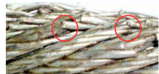
Wire Breakages at Crown
