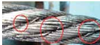
Wire Breakages at Valley
